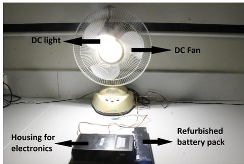
Figure 4: An *UrJar* prototype with DC appliances connected.
